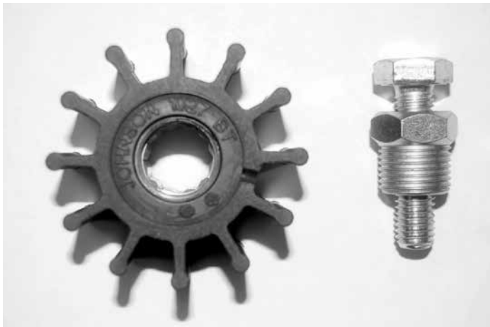
New Yanmar raw water pump impeller, extraction bushing & bolt.
