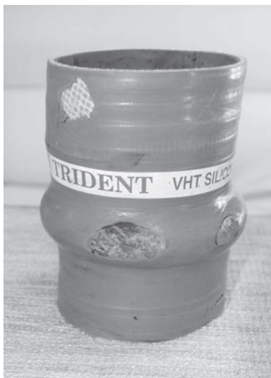
Hump hose showing abraded area that leaked.
