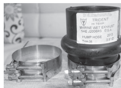
Replacement hump hose and band clamps.
