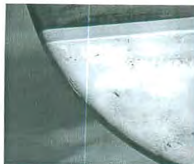
Beckoning bow after soda-blasting damage and vinylester patching
