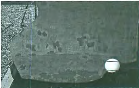
Beckoning keel after soda-blasting damage and initial vinylester repair
