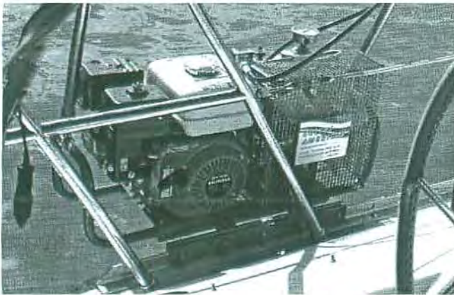
Coltri compressor installed aboard Beckoning... C470 (Hull #76)
