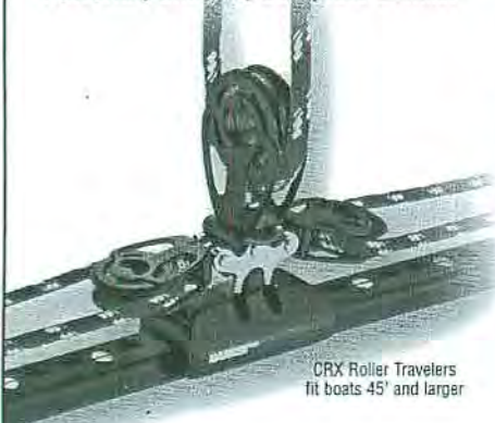
Cars roll on and off track without losing bearings
