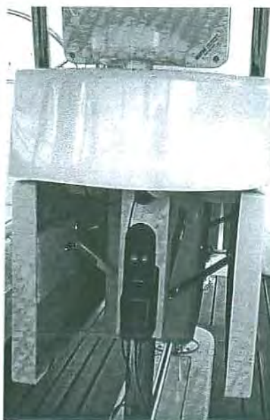
Auto pilot remote for use in foul weather under protection of dodger.
